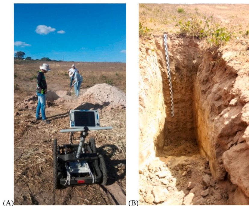
Fig. 3. (A) Ground penetrating radar in the foreground and trench digging for soil description and classification in the background; (B) Soil profile P9 classified as Neossolo Regolítico Eutrófico léptico (Regosols; Psamments). Source: Gustavo M. Vasques.
