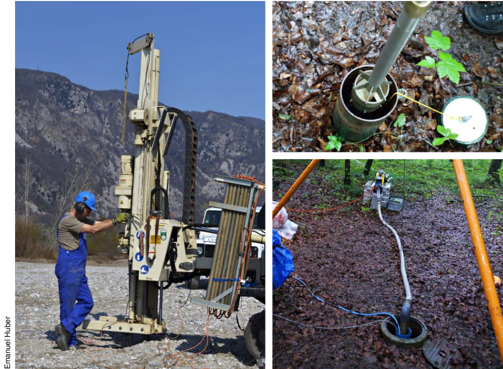
Figure 1.3 – Left: observation well installation with the direct-push technology. Top right: flowmeter measurements. Bottom right: pumping test.
